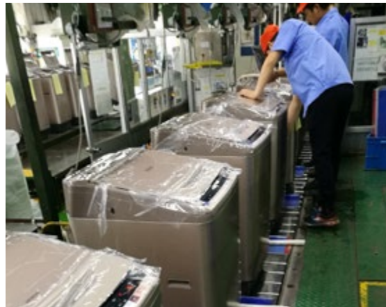
An automatic washing machine acceptance test.
